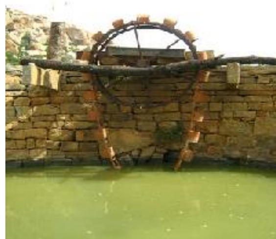
Fig. 7: Persian wheel for water lifting
